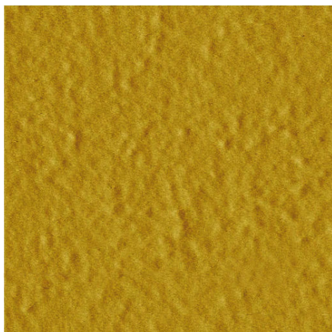
Figure 1. AFM image of PEI adsorbed on the glass surface. A PEI film does not produce nanoring structures (image: 5 \times 5 \mu\text{m} ; z range: 5 nm).
